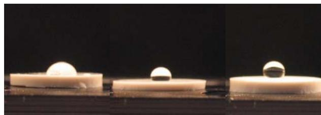
*Fig 3.4: Contact angle images of three pink rubber samples, left to right, flat, big holes, small holes*
