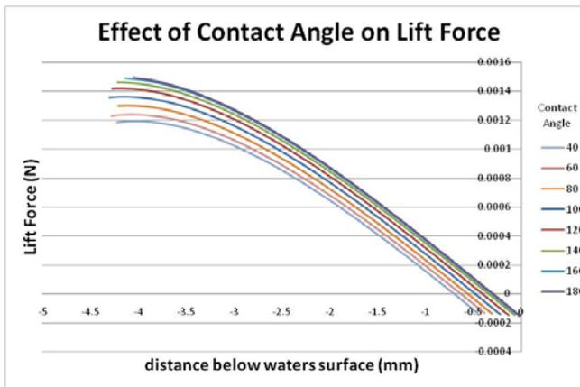
Fig 4.1: The lift force of a .5mm in diameter, 10 mm length of leg without a plastron at various contact angles. Height is distance below initial surface.
