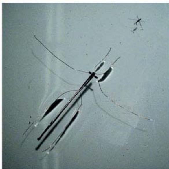
*Fig 1.2: Robostrider, constructed by Hu et al. (2003), notice the real water strider in the upper right hand corner*
