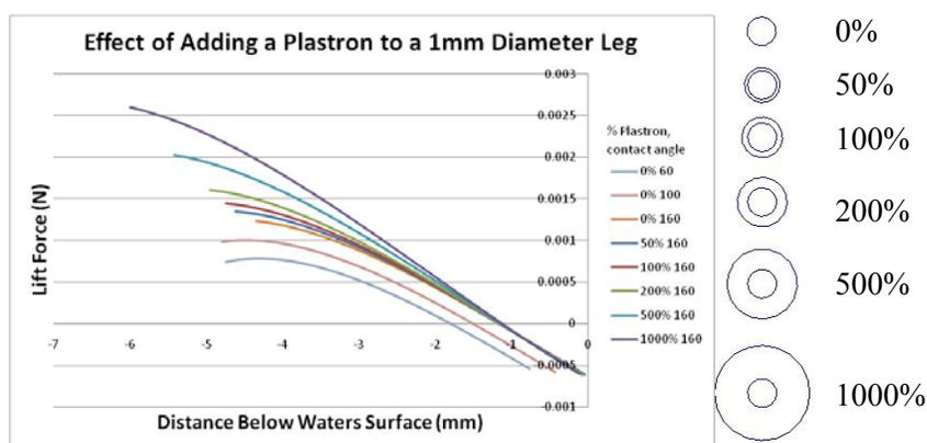
Fig 4.6: Lift force produced by a steel leg with a layer of air surrounding it. This volume of air is a given percent of the volume of the steel also represented by images on the right. The density of the steel was incorporated. Height is distance below initial surface.
