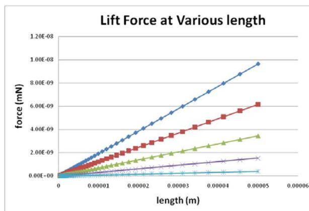
Fig 4.4: The forces produced by a single nano-hole as length increases
