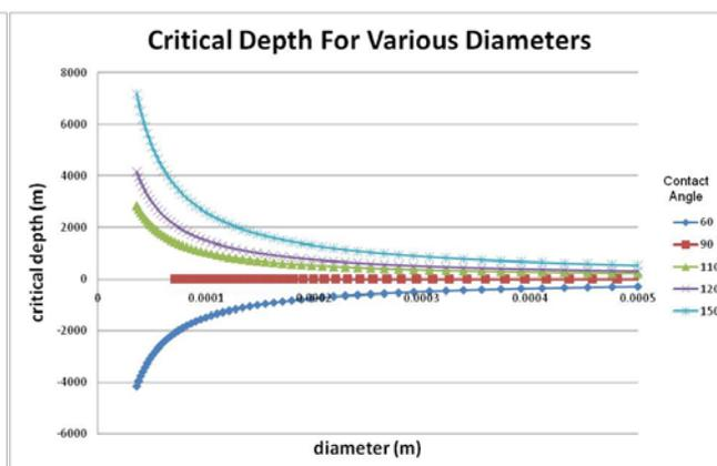
Fig 4.5: The critical depth change based on diameter
