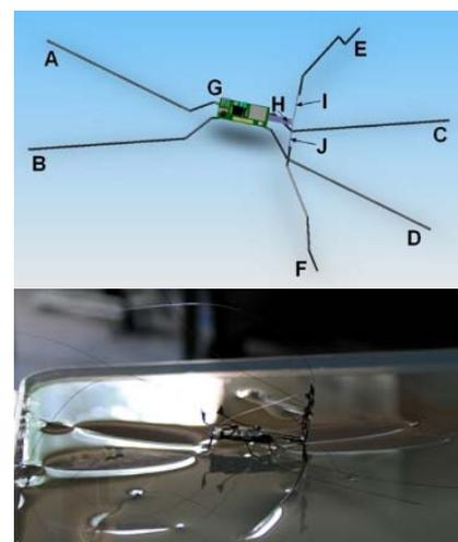
*Fig 1. 3: A CAD rendering and picture of a water strider robot produced by Song et al.(2007)*
