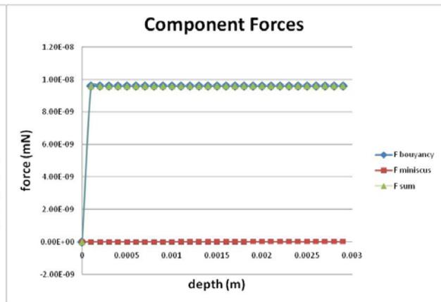
Fig 4.2: The component forces produced by a single nano-hole
