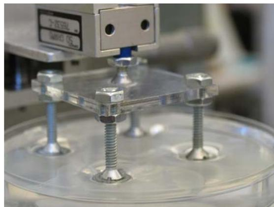
*Fig 3.5: A trial in progress, a load cell measures how much the feet of the stage push back. The stage and load cell are moved by a motorized axis controller attached to the load cell.*
