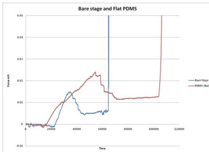
Fig 4.7: Lift force versus time for the bare testing apparatus and a flat PDMS sample (85 trials were conducted)
