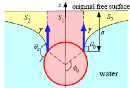
Fig 3.2: 2D model of a wire leg at maximum supportive force  $F_s=2\gamma$  (Suzuki et.al, 2007)
