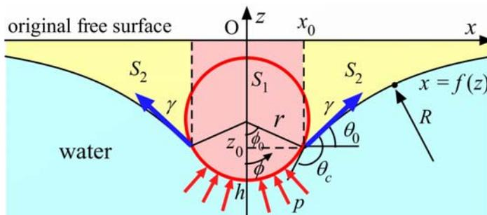
Fig 3.1: A 2D model of a wire supporting leg (Suzuki et.al, 2007)
