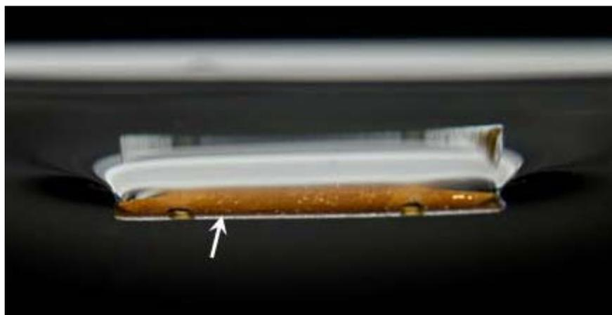
Fig 5.1: Visible plastron on a gold wire constructed by Shi (2007)
