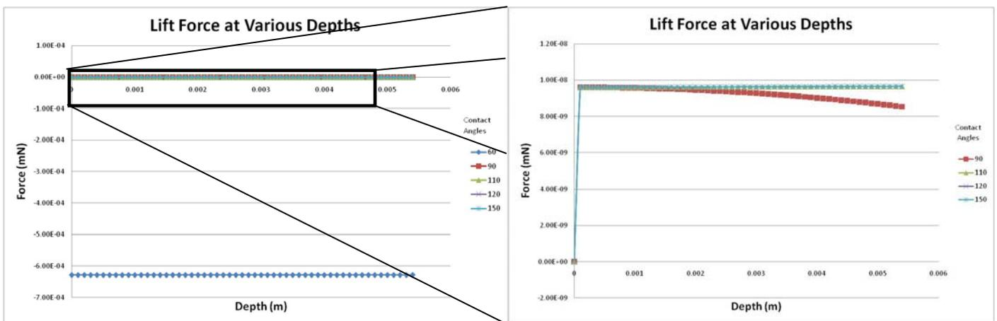
Fig 4.3: The forces produced by a single nano-hole at various depths, graph A (left) shows all the contact angles tested, graph B(right) is the same graph without the 60° contact angle graphed to show more detail.
