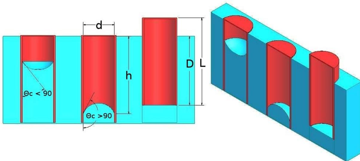
Fig 3.3: Model of nano-holes: nano-holes red, water blue. (Left) nano-hole with a contact angle under  $90^\circ$ , notice that the water climbs up the tube, (Middle) nano-hole with a contact angle greater than  $90^\circ$ , (Right) nano-hole above its critical depth
