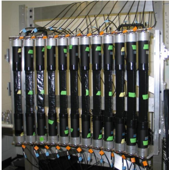
This picture above is an image of ½ of the full array of LENDA. LENDA measures the amount of neutrons that can be emitted at various angles during nuclear reactions. The
