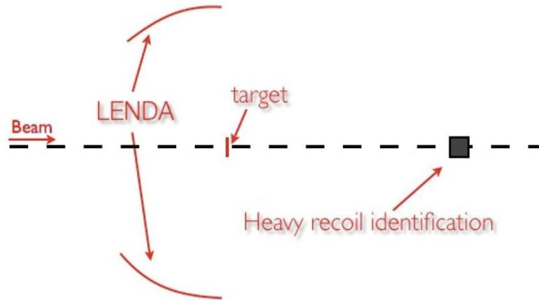
This is the expected setup of LENDA when the actual experiment will be conducted.
