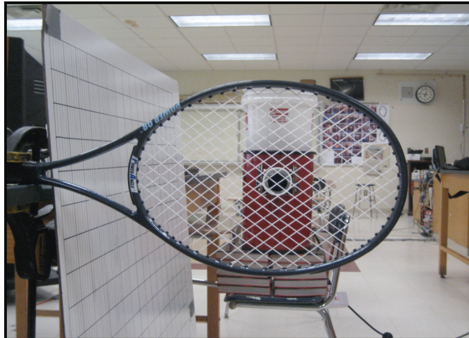
Figure 3.4 The path of the tennis balls projected during the testing of both ball control and power. The tennis balls made contact with each racket exactly 16 cm from the tip, at the “sweet spot,” perpendicular to the strings of the tennis rackets.
