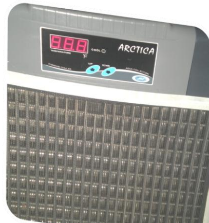
The cooler maintained a constant temperature of approx. 15 degrees Celsius for a stable ecosystem home to living organisms.
