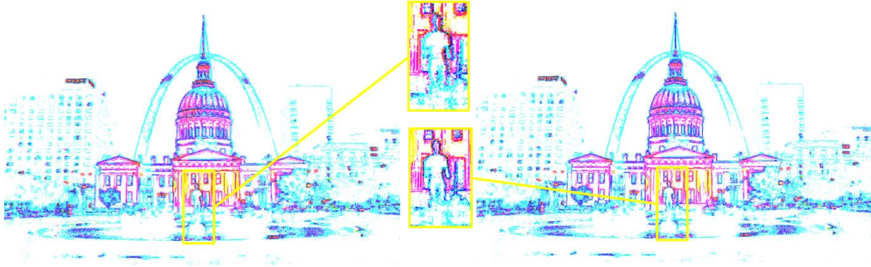
Fig. 4. A comparison between contrast images before and after alignment using the information from cross-correlation. Each color channel shows different LDR image in exposure stack. Left image shows misalignment. For the right image, the third and fourth images in the input sequence moved according to moving vectors found. The right image shows well aligned.
