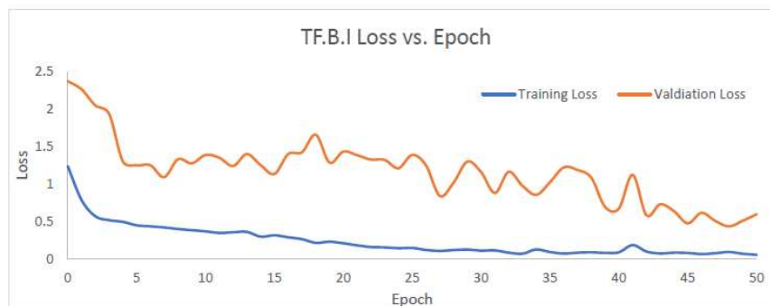
FIGURE 4: Validation loss shows significant downward trend and is converging with training loss. The loss vs. epoch graph provides better insight about the model’s ability to generalize data than Figure 3, as the distance between the validation loss and training loss decreases significantly at the end of training.
