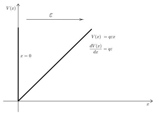
These wells play a significant role in semi-conductor and transistor design. A noteworthy example is the high-electron-mobility transistor (HEMT) which confines electrons to the triangular well produced when different semi-conducting materials are juxtaposed to create a heterojunction.
