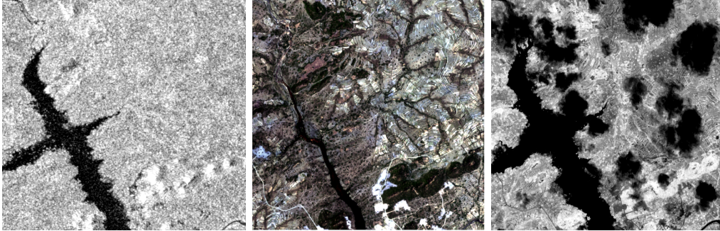
Figure 1: Examples of preprocessed satellite frames. Left: a Sentinel-1 SAR image with visible speckle. Middle: a Sentinel-2 optical image shown in RGB. Right: a grayscale map derived from optical bands using a water index. These examples show why flood detection from satellite images is not the same as ordinary clean-image classification.
